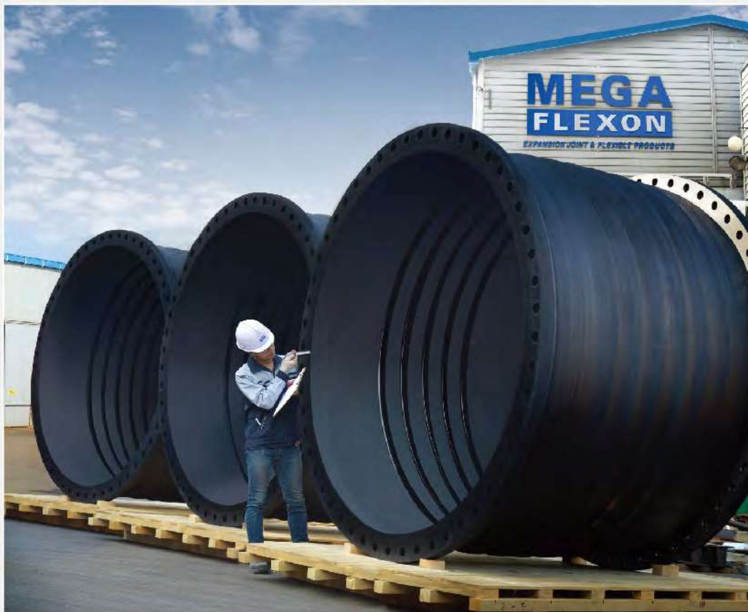
ERGENE SEA OUTFALL PROJECT, TURKEY 87 INCH (DN 2200) x 1800mmL FIVE OPEN ARCH BURIED TYPE
