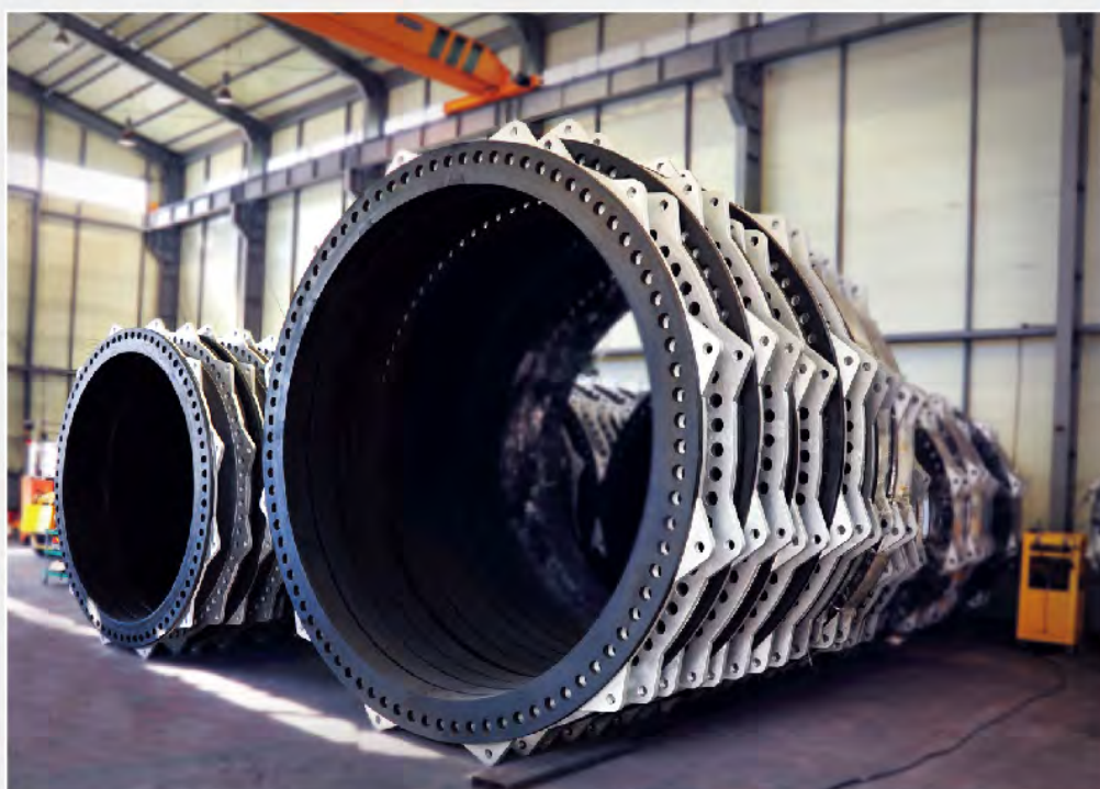
DOOSAN HEAVY INDUSTRIES & CONSTRUCTION CO.,LTD RAS AL KHAIR POWER & DESALINATION - PH.1 160 INCH (DN 4000) X 500mmL SINGLE OPEN ARCH TYPE
