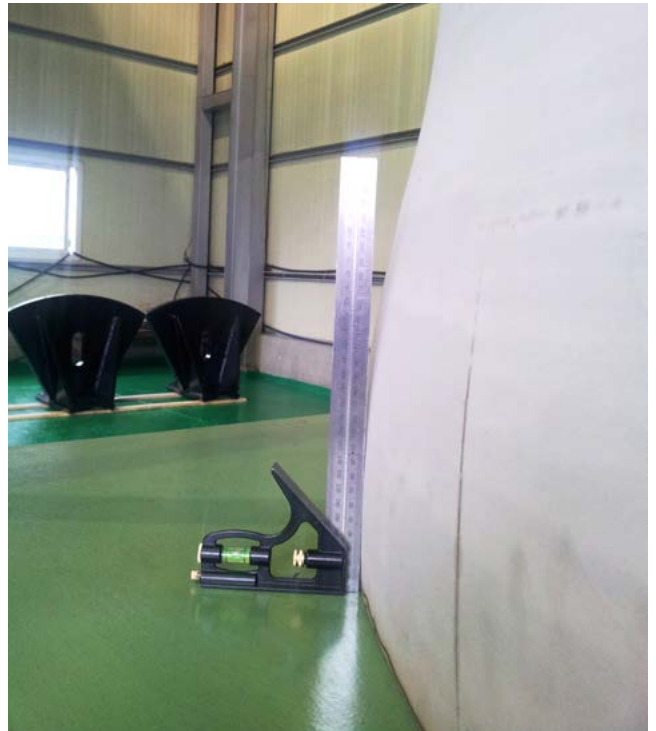
▲ Expanded Pipe View / ASTM A240 TP 321H / 20T 75mm expanded from original diameter 2400mm
