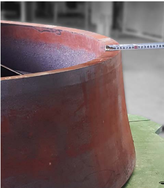
▲ Thickness Measurement (52mm) / ASTM A516 Gr70 50mm expanded from original diameter 1800mm
